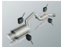
Vibration test of high-temperature-muffler
