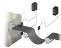
Thickness measurement/loop control of a rubber sheet
